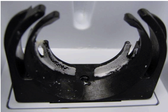
Figure 8-7. Injector Switch Pin with Accumulated Fluid Spillage
