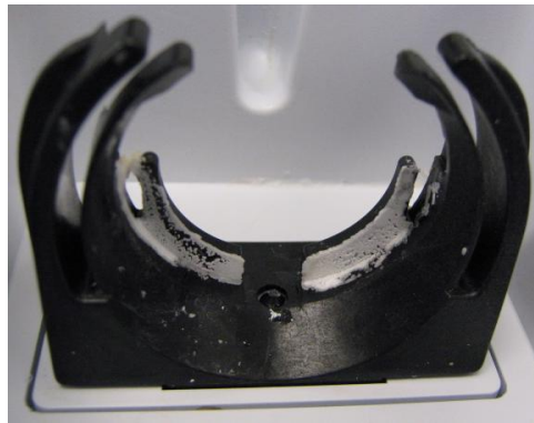
Figure 8-7. Injector Switch Pin with Accumulated Fluid Spillage
