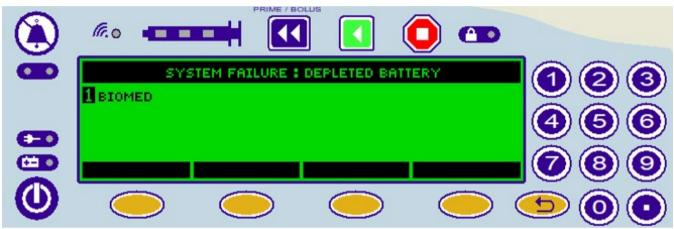
Figure 1: System Failure: Depleted Battery Alarm
