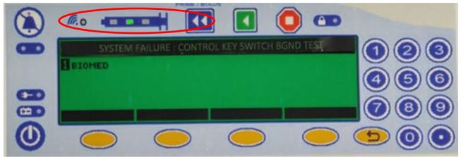
Figure 2: Green light indicates IVOT Infusion Continues after System Failure
