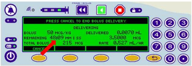
Figure 4: Example of Incorrect Time Remaining. "REMAINING 48:09 MM:SS" should be displayed as "REMAINING 04:09 MM:SS"
