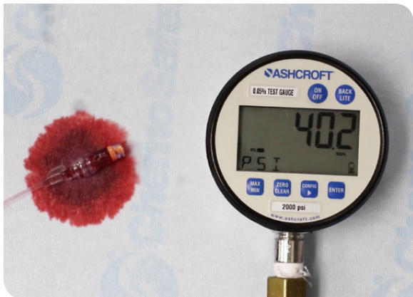
FIGURE 2. NEUTRACLEAR BACK PRESSURE LEAKAGE
