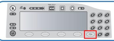
4) If you miss the size on the screen, pressing the back button on the pump will again briefly flash the size of the syringe in the upper left hand corner without stopping the infusion. The screen will then return to the normal run screen.
