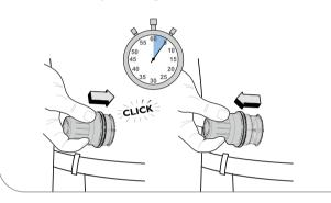
8. Connect tubing and fill according to pump user manual.\*
