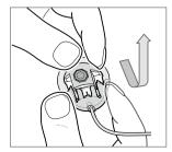
Open the connector by pinching the site connector arms inward and sliding fully open.
