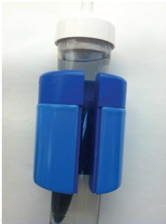
Illustration 11- Proper sensor placement
